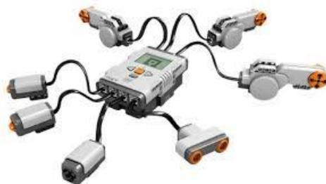
**Figura 8. Lego Mindstorms NXT (Lego, 2009) (a) CPU. (b) sensor de toque. (c) sensor de som. (d) sensor de luz. (e) sensor ultra-sônico. (f) servo-motor**
