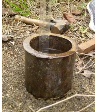
Figura 23: Infiltrômetro de Hills.
