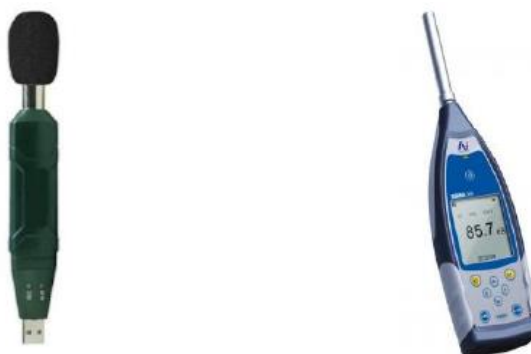
FIGURA 54 - SOUND LEVEL DATALOGGER EXTECH 407760 E SOUND LEVEL METER BSWA TECH 308, RESPECTIVAMENTE.
