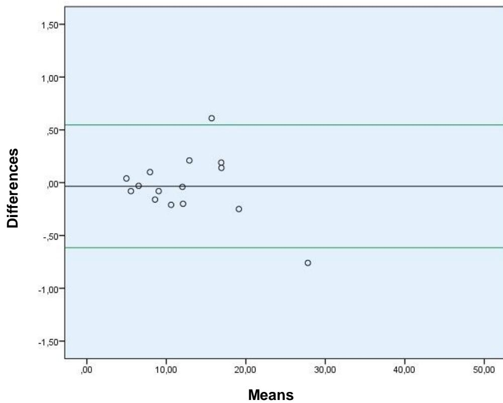
**Figure2.** Bland-Altman plot for compass and digital caliper measurements from operator 1. The center line represents the mean of the differences and the upper and lower green line represent the 95% confidence interval limits.
