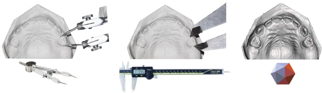
**Figure 1.** A- Compass measurements; B- Digital caliper measurements; C- Digital measurements.
