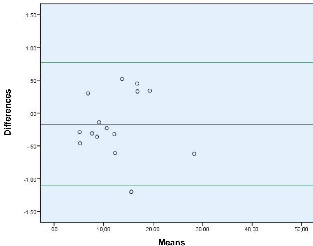
**Figure3.** Bland-Altman plot for compass and digital caliper measurements from operator 2. The center line represents the mean of the differences and the upper and lower green line represent the 95% confidence interval limits.
