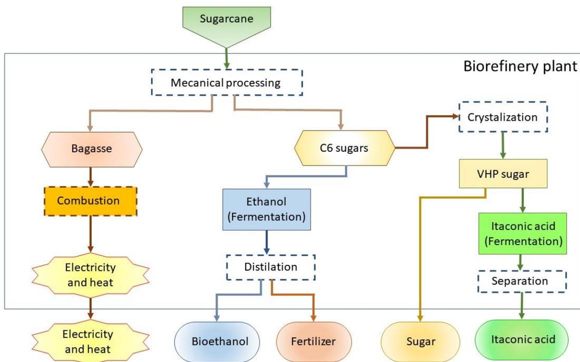
**Figure 7.26** Proposal of a 4-platform biorefinery (C6 sugars, bagasse, electricity & heat, itaconic acid) biorefinery using sugarcane for bioethanol, electricity, heat, sugar, fertilizer and itaconic acid (adapted from IEA Bioenergy (2013)).
