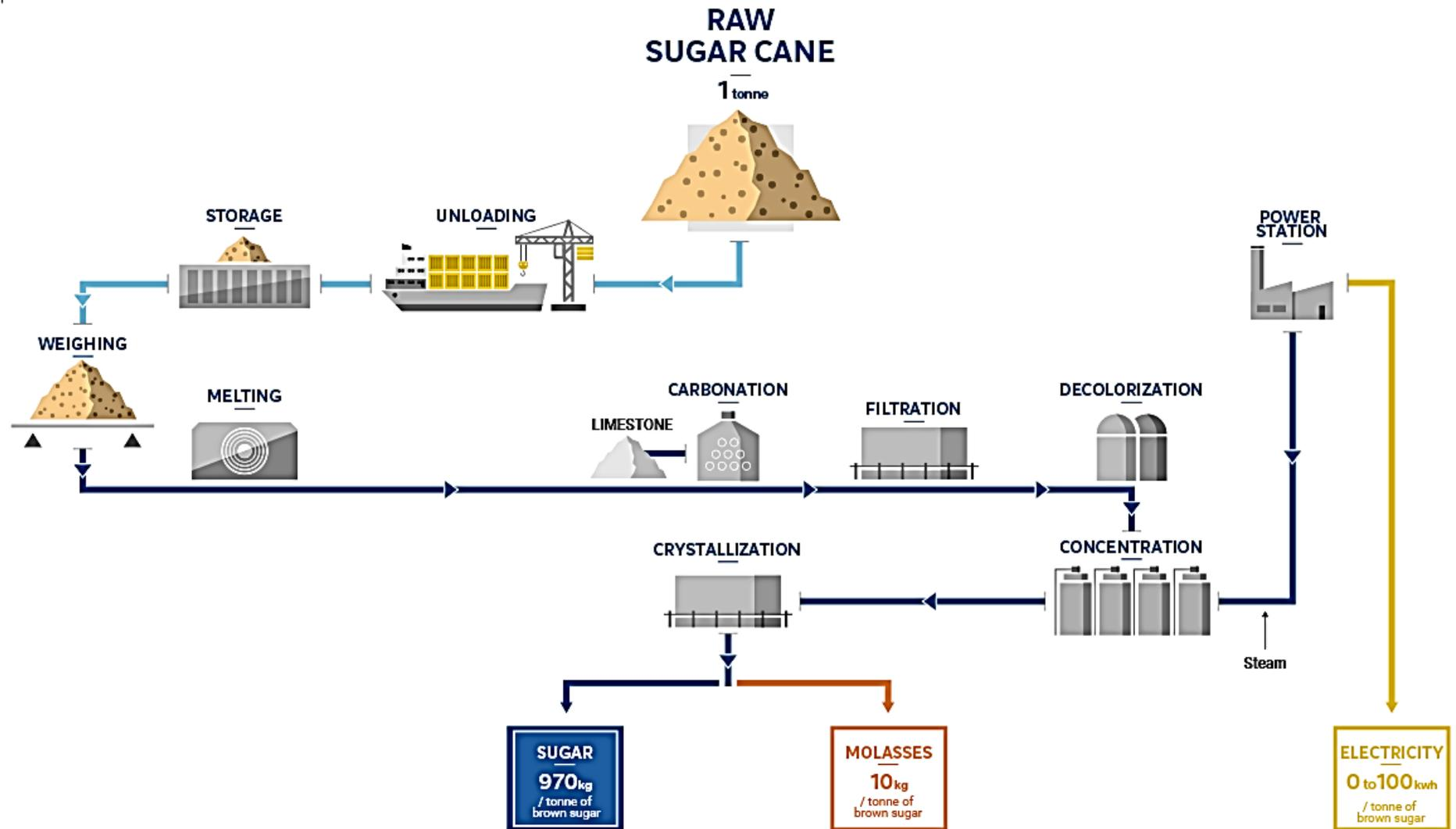
Figure 3.3 Simplified flow diagram of refined sugar, molasse and electricity production at a sugar refinery (SUCDEN 2017a).
