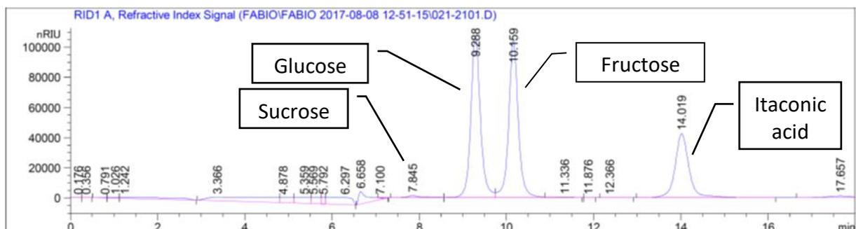
**Figure 6.2** Chromatogram of the peaks of IA, sucrose, glucose and fructose with refractive index detection.
