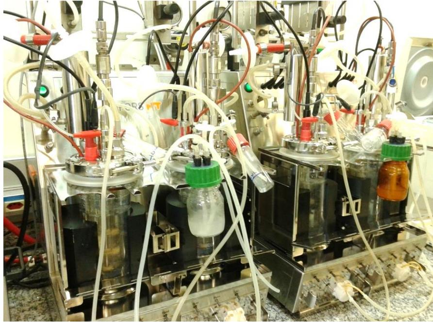
**Figure 6.1** Bioreactor Multifors 2 incubated with *A. terreus* NRRL 1960.
