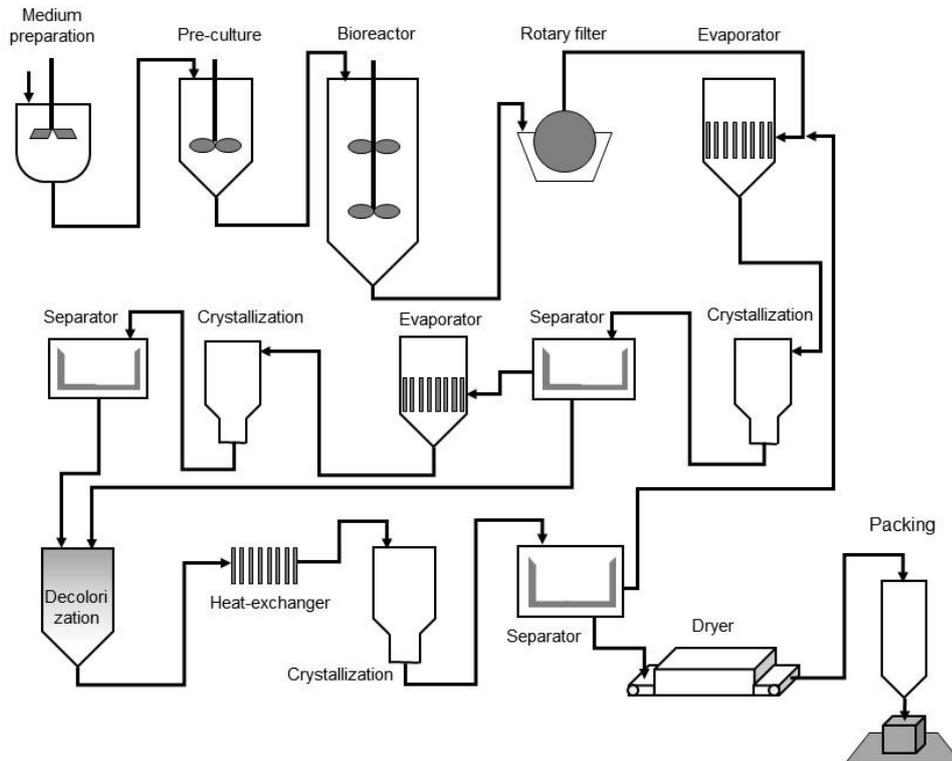
**Figure 2.6** Diagram of itaconic acid production by *A. terreus* (adapted from Okabe et al. (2009)).
